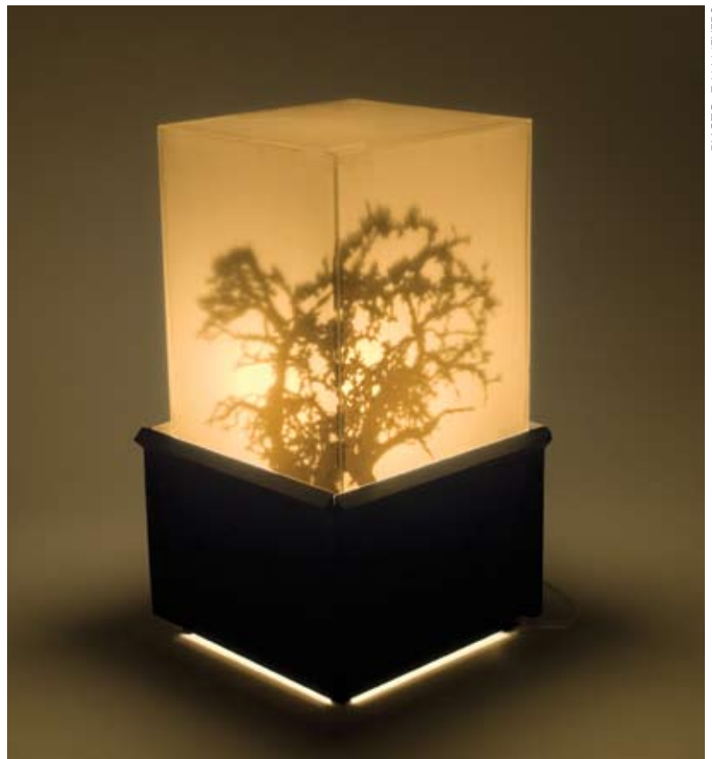
Designed by Huei-Ting Wu, this adaptation of an existing lighting fixture was inspired by a traditional Japanese table lamp. Wu was interested in using man-made materials to create an object with a natural character. It measures 16" high x 10" wide x 10" deep and is composed of sanded clear acrylic, tinted laser-cut acrylic panels, and stained plywood. A 20-watt, self-ballasted compact fluorescent provides the illumination.
